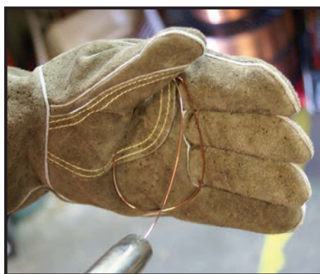
(8) A simple check for the correct drive tension is to bend the end of the wire over hold it about 4" from your hand and let it run into your hand, it should coil round in your hand without stopping and slipping at the drive rollers, increase the tension if it slips.
