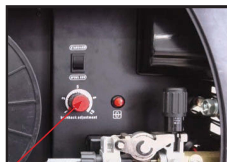
(17) Adjust the burn back control to prevent the wire sticking in the weld pool.
