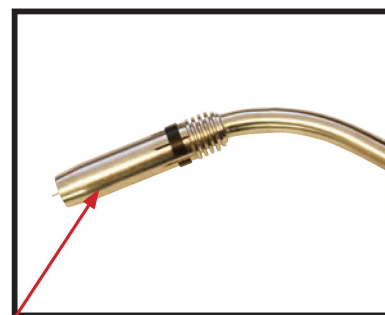
(11) Remove the gas nozzle and contact tip from the front end of the mig torch. NB: Torch ends differ according to Machine!
