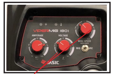
(17) Set welding parameters using the voltage and wire feed controls.
