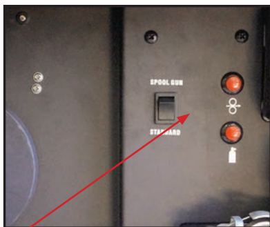
(1) Set Standard/Spoolgun selector switch inside door to Spoolgun
