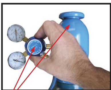
(15) Carefully open the valve of the gas cylinder, set the flow to 20-25 CFH
