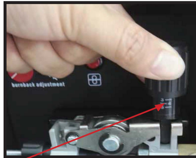
(9) Close down the top roller bracket and clip the pressure arm into place. NOTE: MIG 180 is not geared
