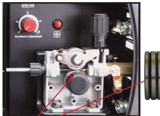
(6) Fit the correct sized Knurled Drive roller for Gas Less Flux Cored wire NOTE: MIG 180 not geared
