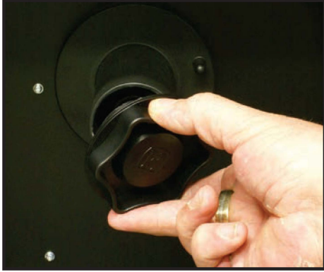
(1) Remove the spool retaining nut.
