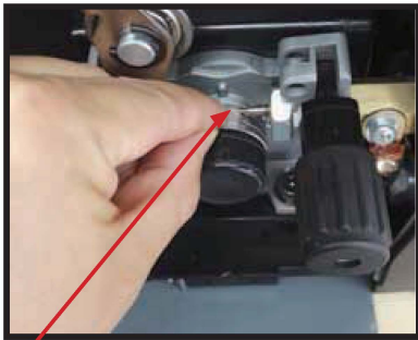
(8) Feed wire over the drive roller into the outlet guide tube, Push the wire through approx 6". Use a Knurled Drive Roller of the correct size NOTE: MIG 180 not geared
