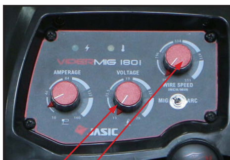
(16) Set welding parameters using the voltage and wire feed controls.
