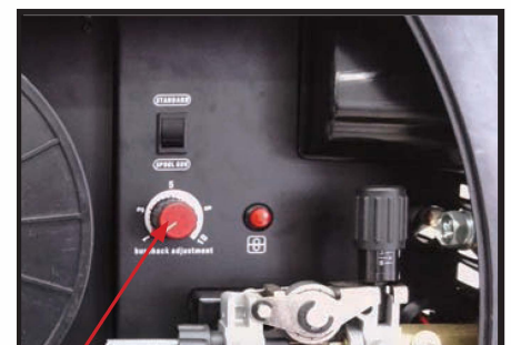
(16) Adjust the burn back control to prevent the wire sticking in the weld pool.
