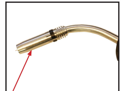
(15) Fit the nozzle to the torch neck ready for welding.
