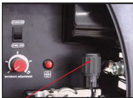
(10) Apply a medium amount of pressure to the drive roller
